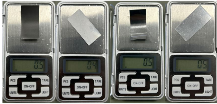
Figure 4: samples lined up after coating showing their mass, left to right: FeCu, Tio2, Graphene, Control
