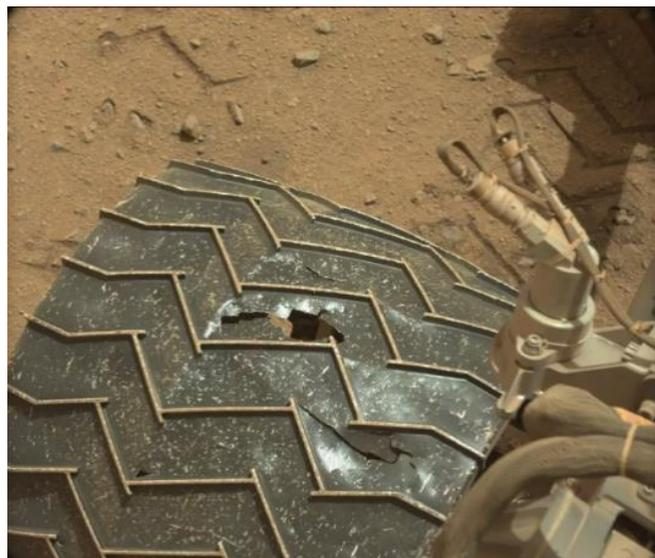
Figure 6: The damage to the Curiosity's aluminum wheel caused by Mars dust.
