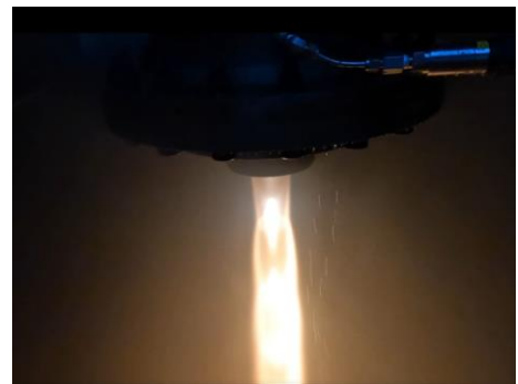
Fig. 9. Thrust Vector Control Hot-firing Test
