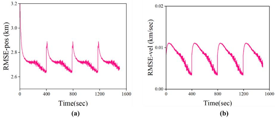
**Fig.8.** RMSE in position and velocity estimates using multi-sensor data fusion.
