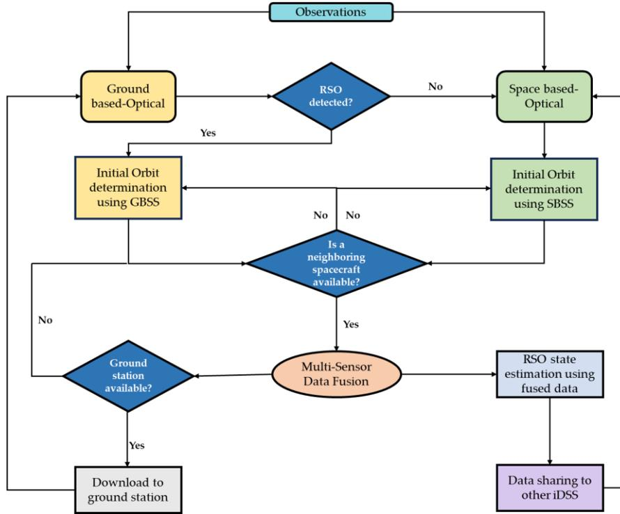
Fig.2. RSO tracking algorithm flowchart.
