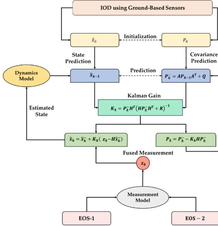
Fig.4. Multi-sensor data fusion algorithm.
