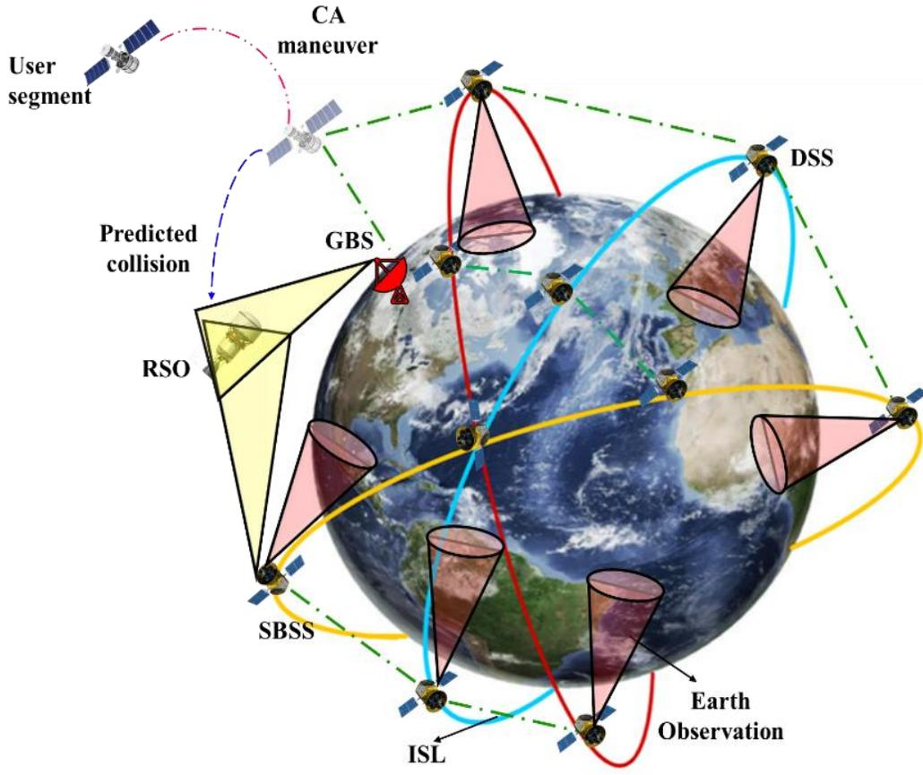
Fig.5. RSO tracking using hybrid sensor networks mission scenario.
