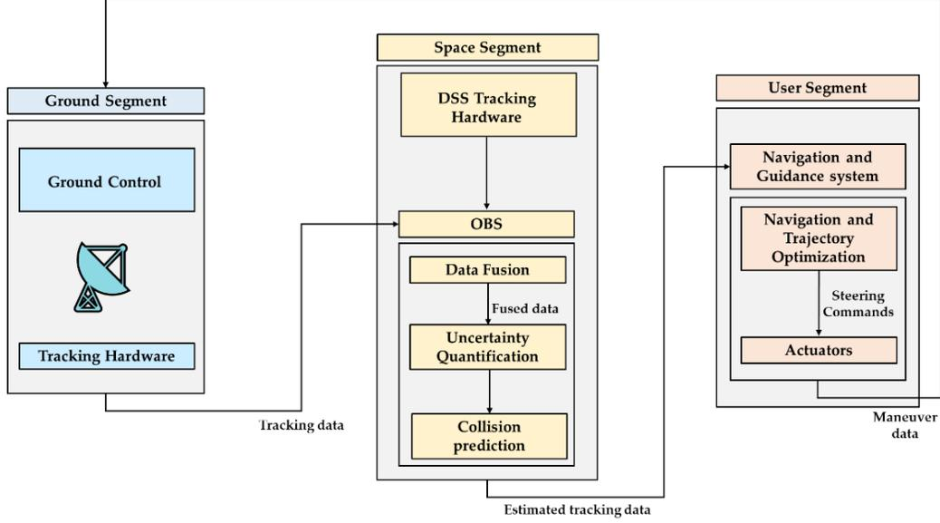
Fig.6. Autonomous tracking system architecture.
