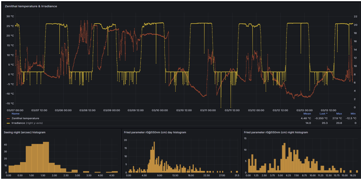
FIG. 4: Example of data from the weather station dashboard: Zenithal temperature, irradiance, atmospheric seeing resolution, and Fried parameter r_0 .
